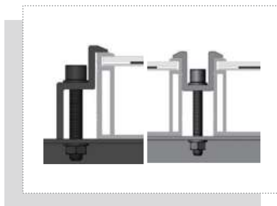
Installation of end clamp and middle clamp
