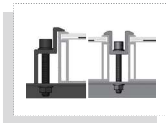
Installation of end clamp and middle clamp
